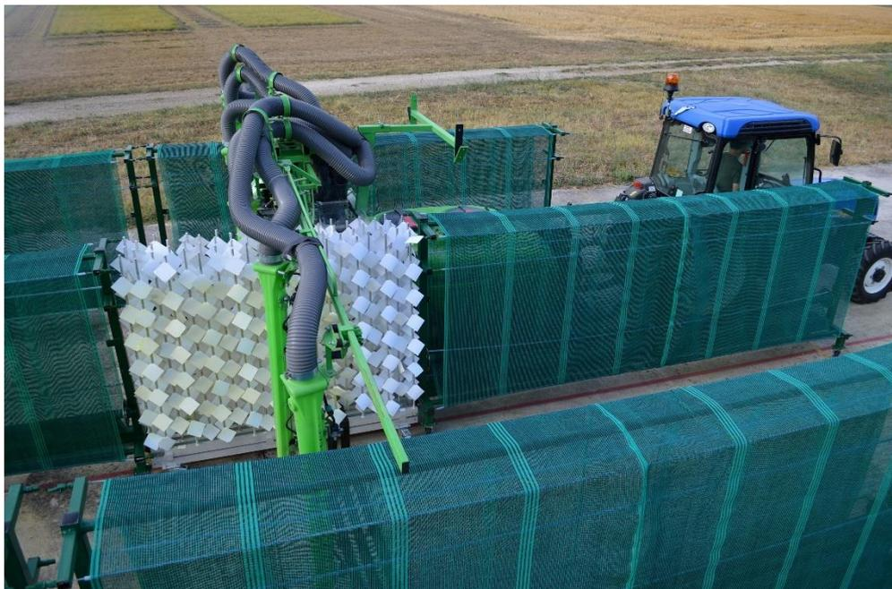
Photo n° 21 : banc Evasprayviti en configuration Vigne Semi-Large (Source IFV)
